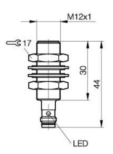
**Inductive Sensors** BES 516-370-G-E5-Y-S 49 M12x1 x 44 normally-closed Sn=4mm shielded
